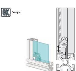
Holes are tapped on a bracket for cover mounting
