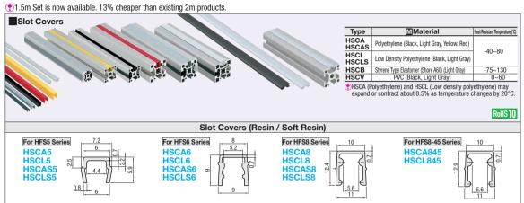
Slot covers are used in reverse as Plate Covers, HES5 can hold a 3mm plate, HES6, HES8 and HES8-45 can hold a 5mm plate. \*\* HSCL (soft resin) is made of softer material compared to HSCA (resin). Post assembly insertion is easy. (For details, see lower section of P.773.)
