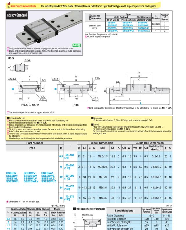
Pair Variation of Width W2 20 10 Running Parallelism of Plane C against Plane A See P. 525 Running Parallelism of Plane D against Plane A Slight Clearance Type has clearance (Gap) between rails and blocks.
