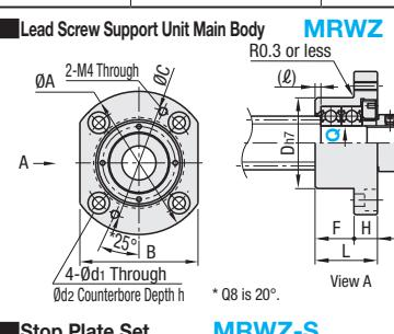
Lead Screw Support Unit Main Body
