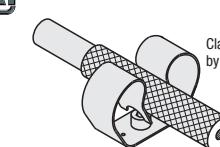
Clamping force may be adjusted slightly by tightening the mounting screw.
