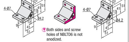
Both sides and screw holes of NBLTD6 is not anodized.
