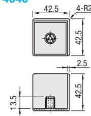
■ The pin shape and numbers of extrusion caps may be changed to prevent caps from easily falling off. ■ Material: Polyamide
