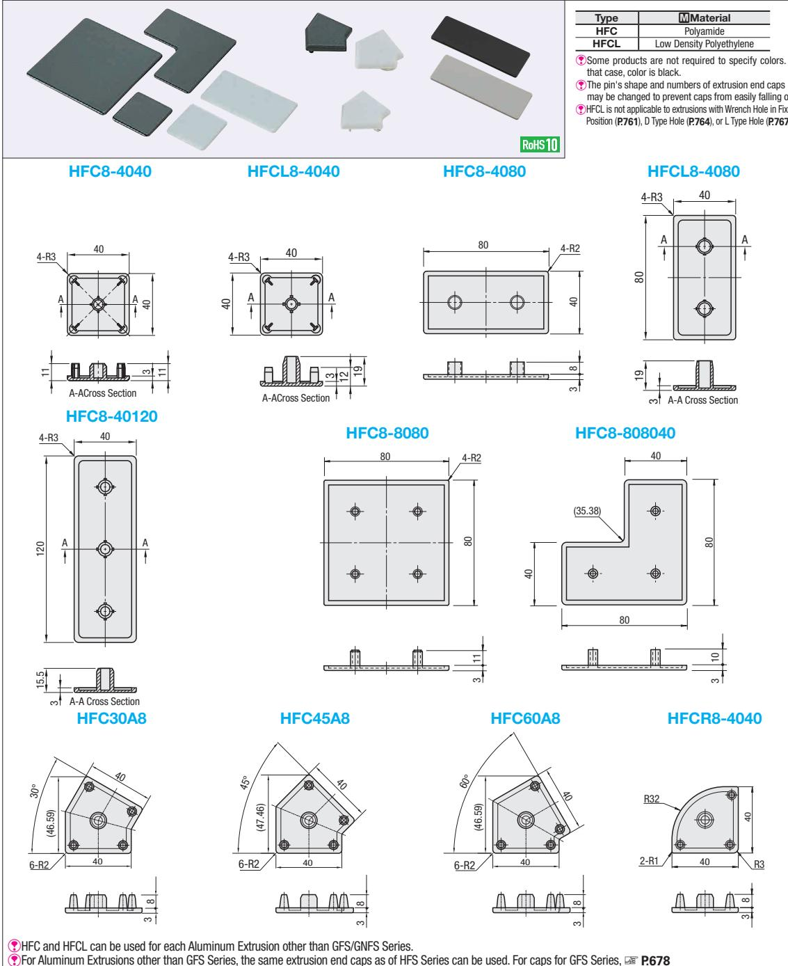
■ HFC and HFCL can be used for each Aluminum Extrusion other than GFS/GNFS Series.
