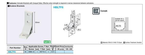
Features: Numbers of screws are the same as HBLTS8-45. Extrusions can be connected more securely.
