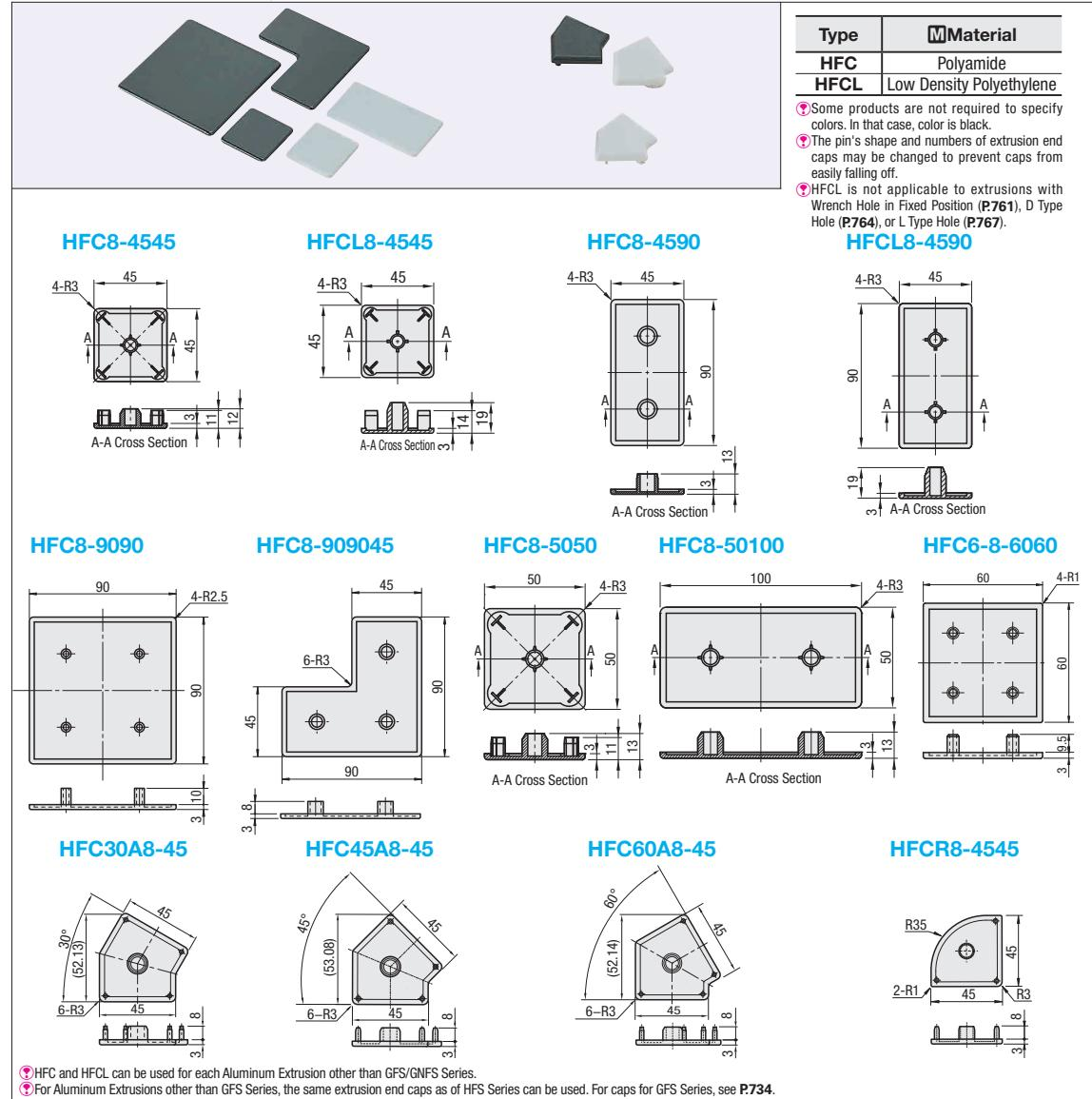
■ HFC and HFCL can be used for each Aluminum Extrusion other than GFS/GNFS Series.
