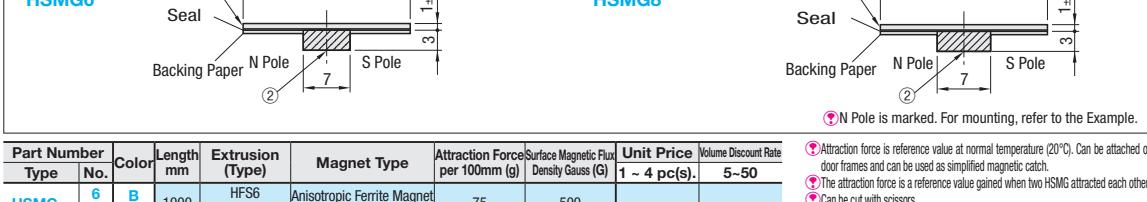
Attraction force is reference value at normal temperature (20°C). Can be attached on door frames and can be used as simplified magnetic catch.
