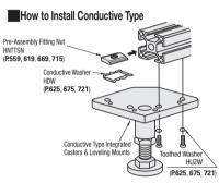
Conductive washers and toothed washers are not included with Conductive Type.
