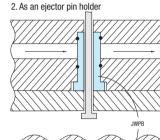
Process the inner diameter according to the ejector pin size for application method no. 2. Also process the outer diameter to reduce cooling water pressure drop.
