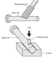
Normally, it is quite easy to file down an ejector pin using a regular file (metalworking file).
