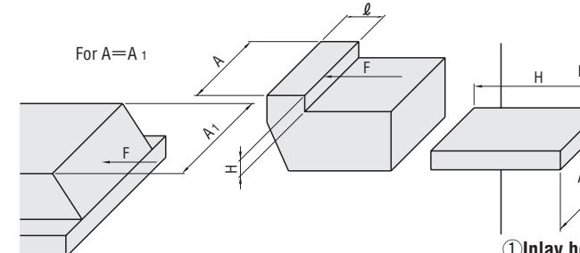
Considering the force acting on the inlay section to be cantilever
