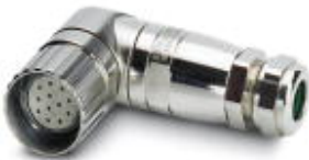
M23 socket, 12-pos., angled, freely configurable, with solder connection, for external cable diameter of 8 mm ... 12 mm
