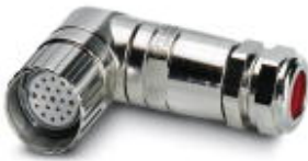
M23 socket, 19-pos., angled, freely configurable, with solder connection, for external cable diameter of 10 mm ... 14 mm
