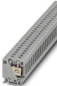
Feed-through terminal block, Connection method: Screw connection, Cross section: 0.2 mm 2 - 2.5 mm 2 , AWG: 24 - 14, Width: 5.2 mm, Color: gray, Mounting type: NS 15
