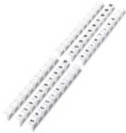
Marker pin Zack strip, Strip, white, Unlabeled, Can be labeled with: Plotter, Mounting type: Plug in, For terminal block width: 6.2 mm, Lettering field: 4 x 4 mm
