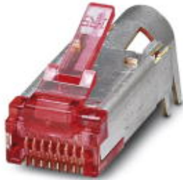
RJ45 male insert, CAT6, 8-pos., shielded, IDC pierce connection, for AWG 27 litz wires ... 24, with strain relief
