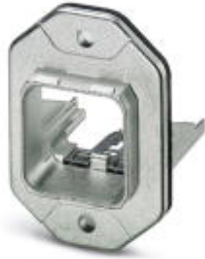
RJ45 panel mounting frame, IP67, for push-pull interlocking, metal, with the Freenet system, for square panel cutout, with grommet, without mounting screws
