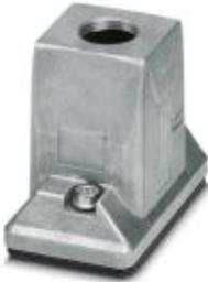
HEAVYCON ADVANCE sleeve housing, B6, with stainless steel screw locking (Allen screw), salt-water-resistant aluminum, height 74 mm, with 1x M20 thread, straight cable outlet, without surface; conductive seal (EMC properties)
