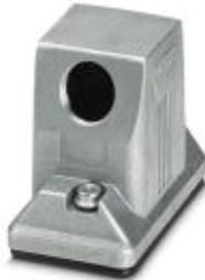
HEAVYCON ADVANCE sleeve housing, B6, with stainless steel screw locking (Allen screw), salt-water-resistant aluminum, height 74 mm, with 1x M20 thread, lateral cable outlet, without surface; conductive seal (EMC properties)
