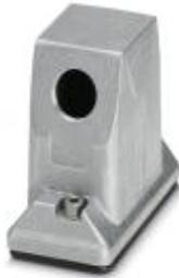
HEAVYCON ADVANCE sleeve housing, B10, with stainless steel screw locking (Allen screw), salt-water-resistant aluminum, height 93.7 mm, with 1x M32 thread, lateral cable outlet, without surface; conductive seal (EMC properties)
