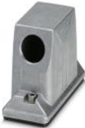
HEAVYCON ADVANCE sleeve housing, B16, with stainless steel screw locking (Allen screw), salt-water-resistant aluminum, height 93.7 mm, with thread, 1 x M32 lateral cable outlet, without surface; conductive seal (EMC properties)
