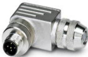
Bus system plug, plug angled, 5-pos., M12 shielded, gold-plated contacts, B-coded, screw connection, metal knurl, cable gland Pg9
