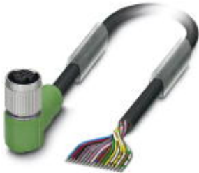
Sensor/Actuator cable, 17-position, PUR halogen-free, Black RAL 9005, Free cable end, on Socket angled M12 SPEEDCON, A-coded, Cable length: 1.5 m
