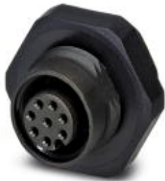
Sensor/actuator flush-type connector, socket, 8-pos., M12, A-coded, rear/screw mounting with Pg9 thread, with solder cups, plastic version
