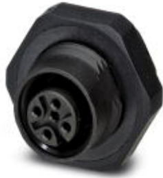
Sensor/actuator flush-type connector, socket, 5-pos., M12, A-coded, rear/screw mounting with Pg9 thread, with straight solder connection, plastic version
