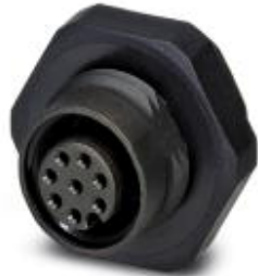
Sensor/actuator flush-type connector, socket, 8-pos., M12, A-coded, rear/screw mounting with Pg9 thread, with straight solder connection, plastic version
