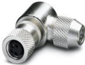
Sensor/actuator connector, socket, angled, 4-pos., M8, shielded, solder connection, metal knurl, cable diameter max. 5 mm
