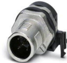
Sensor/actuator flush-type connector, connector, 5-pos., M12 SPEEDCON, A-coded, rear/screw mounting with M12 thread, with polarity protection, with angled solder connection
