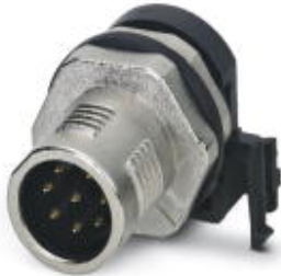
Sensor/actuator flush-type connector, connector, 8-pos., M12 SPEEDCON, A-coded, rear/screw mounting with M12 thread, with polarity protection, with angled solder connection
