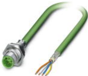
Bus system flush-type plug, PROFINET, 4-pos., M12, shielded, D-coded, SPEEDCON, rear/screw mounting with Pg9 thread, with 2.0 m bus cable, 2 x 2 x 0.34 mm 2
