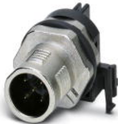
Sensor/actuator flush-type connector, connector, 5-pos., M12 SPEEDCON, A-coded, shielded, rear/screw mounting with M12 thread, with polarity protection, with angled solder connection
