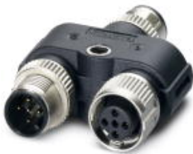
Y distributor, 5-position, shielded, Plug straight M12 SPEEDCON, A-coded, on Socket straight M12 SPEEDCON, A-coded and Plug straight M12 SPEEDCON, A-coded
