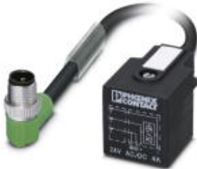
Sensor/Actuator cable, 3-position, PUR halogen-free, Black-gray RAL 7021, Plug angled M12, A-coded, on Valve connector A, with 1 LED, connected with Z diode, Cable length: 1.5 m
