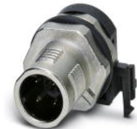
Sensor/actuator flush-type connector, connector, 4-pos., M12 SPEEDCON, A-coded, shielded, rear/screw mounting with M12 thread, with polarity protection, with angled solder connection
