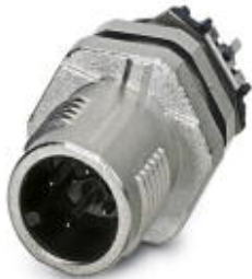
Sensor/actuator flush-type connector, connector, 4-pos., M12 SPEEDCON, shielded, A-coded, rear/screw mounting with M12 thread, with straight THR solder connection
