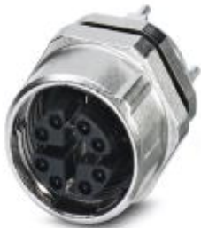
Flush-type socket, CAT6 A , Ethernet, 8-pos., M12 SPEEDCON, rear/screw mounting with M12 fastening thread, with straight solder connection
