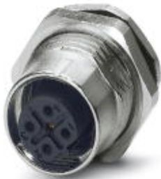
Sensor/actuator flush-type socket, 5-pos. with shield contact, M12 SPEEDCON, B-coded, rear/screw mounting with M16 thread, with straight solder connection
