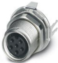
Sensor/actuator flush-type connector, socket, 6-pos. M8, rear/screw mounting with M10 fastening thread, with straight solder connection
