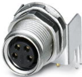
Sensor/actuator flush-type connector, socket, 4-pos. M8, rear/screw mounting with M10 fastening thread, with angled solder connection
