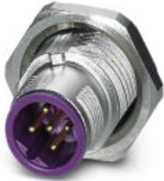
Sensor/actuator flush-type plug, with violet contact carrier, 5-pos., M12 SPEEDCON, shielded, B-coded, rear/screw mounting with M16 thread, with straight solder connection
