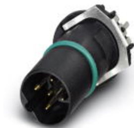
Sensor/actuator flush-type plug, 5-pos., B-coded, with straight THR solder connection, only contact insert
