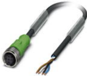
Sensor/Actuator cable, 4-position, PUR halogen-free, Black-gray RAL 7021, Free cable end, on Socket straight M12, A-coded, Cable length: 20 m
