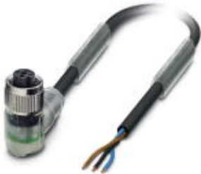
Sensor/Actuator cable, 3-position, PVC, Black RAL 9005, Free cable end, on Socket angled M12, A-coded, with 2 LEDs, Cable length: 8 m
