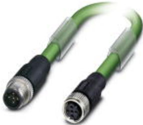
Bus system cable, INTERBUS, INTERBUS, 5-position, PUR halogen-free, Green RAL 6017, shielded, Plug straight M12, B-coded, on Socket straight M12, B-coded, Cable length: 1 m
