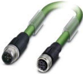
Bus system cable, INTERBUS, INTERBUS, 5-position, PUR halogen-free, Green RAL 6017, shielded, Plug straight M12, B-coded, on Socket straight M12, B-coded, Cable length: 10 m
