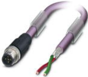
Bus system cable, PROFIBUS, PROFIBUS, 2-position, PUR halogen-free, Violet, RAL 4001, shielded, Plug straight M12, B-coded, on Free cable end, Cable length: 5 m
