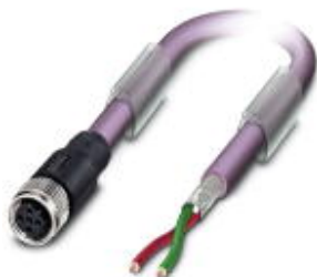
Bus system cable, PROFIBUS, PROFIBUS, 2-position, PUR halogen-free, Violet, RAL 4001, shielded, Free cable end, on Socket straight M12, B-coded, Cable length: 10 m
